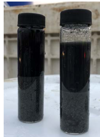
40 mL VOAs filled with soil collected at 15 and 18 ft bgs
