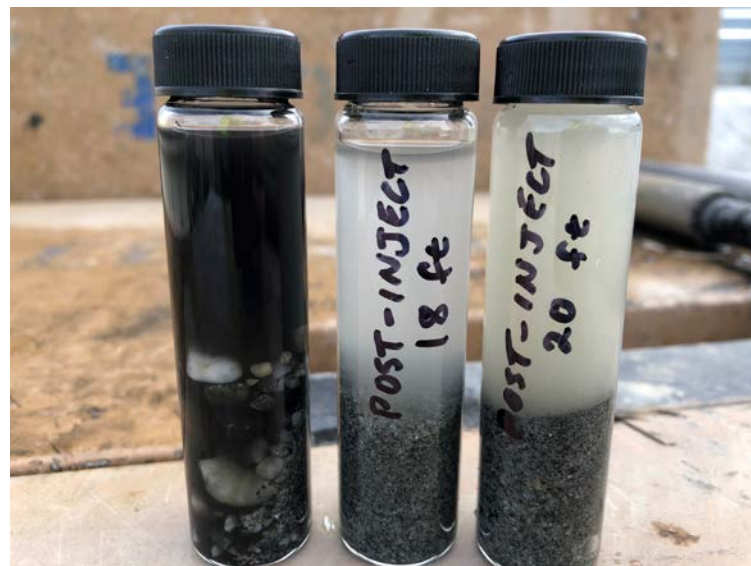
40 mL VOAs filled with soil collected at 15, 18, and 20 ft bgs
